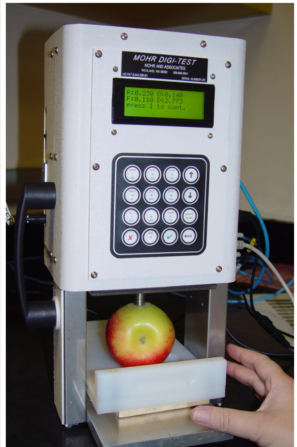
Figure 2. Evaluating crispness with a Mohr Digi-Test.
